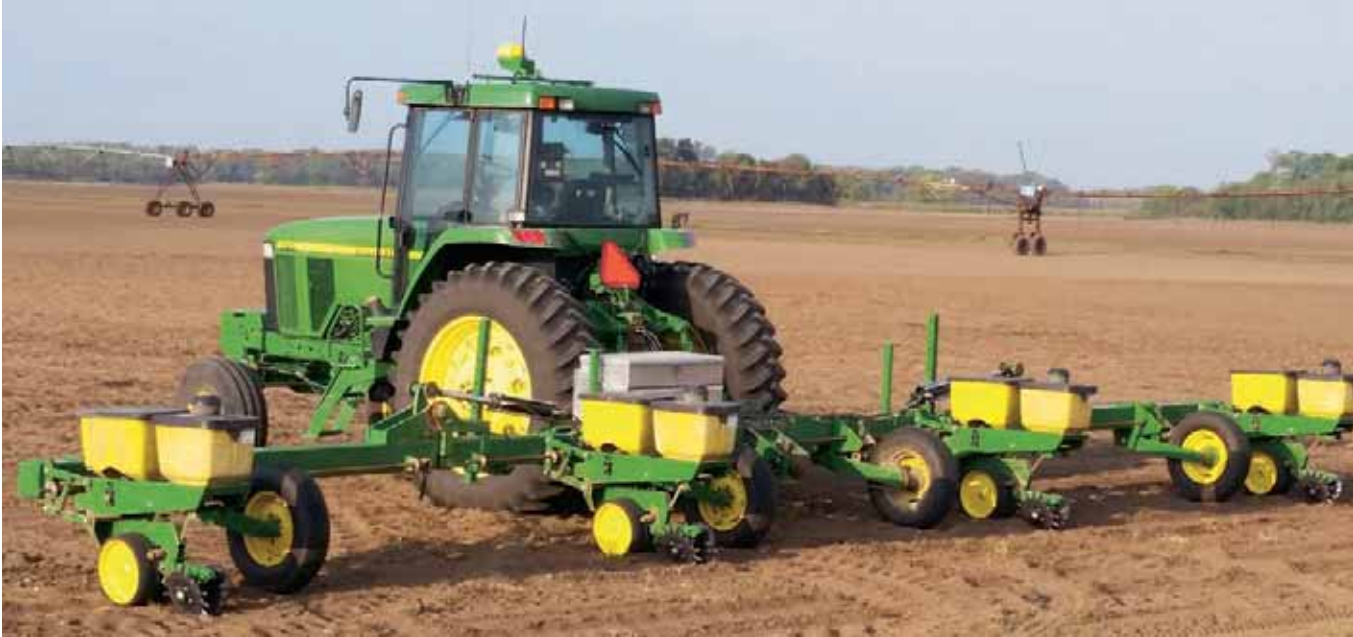
A specialized male row planter for the new wide row production system. GPS allows the male to be planted before or after the female rows.
