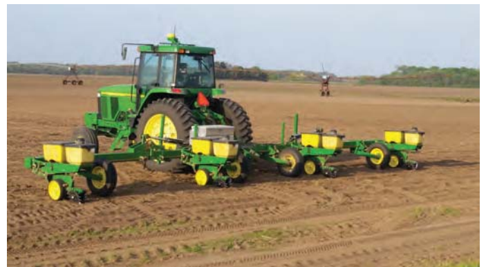
A specialized male row planter for the new wide row seed corn production system. GPS allows the male to be planted before or after the female rows.
